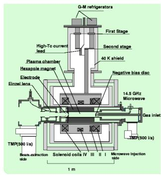
Figure 2: The RAMSES 18 GHz ECR ion source.
