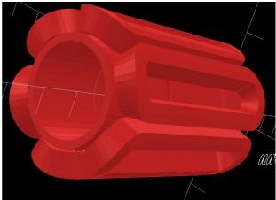
Figure 4 – The innovative design of the SECRAL source magnets at IMP, Lanzhou.
