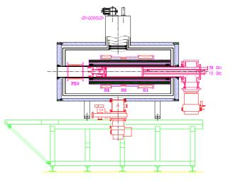
Figure 7: A sketch of the GyroSERSE source.
