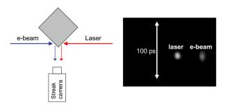
Figure 3: E-beam to laser synchronization measurement.
