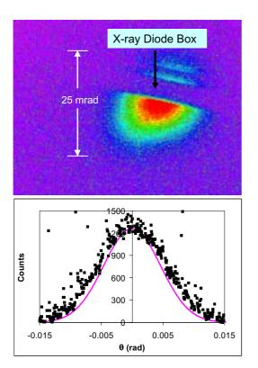
Figure 4: Measurement of X-ray beam profile. Top: CCD image. Bottom: Line-out intensity profile: measurement (dots), theory (line).
