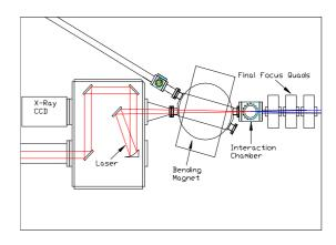
Figure 1: Interaction Geometry
