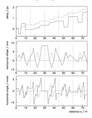
Figure 3: Calculated delay, horizontal offset and angle for an electron with energy deviation  $\Delta E/E = 0.01$  as function of distance from the modulator. For comparison, the dashed lines show the same functions for a modulator in a dispersion-free region. Each vertical line marks the center of a straight section.
