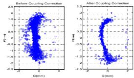
Figure 3: Poincaré surface of the section in the resonant processing frame derived from (x, x') and (y, y'), where  $Q = \sqrt{2J_1\beta_x}\cos\phi_1$ ,  $P = \sqrt{2J_1\beta_x}\sin\phi_1$ . The overall coupling phase is 15° and 90° to have the upright cross section before and after correction, respectively.
