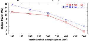
Figure 2: Output power sensitivity to energy spread.
