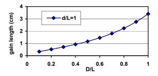
Figure 8. Gain length as a function of D/L, when d/L=1.
