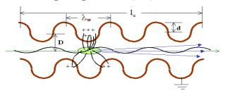
Figure 1. Schematic drawing of image charge undulator.
