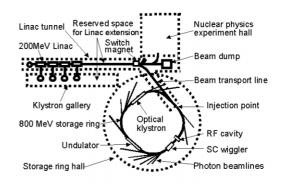
Fig. 1 Layout of Hefei synchrotron radiation source
