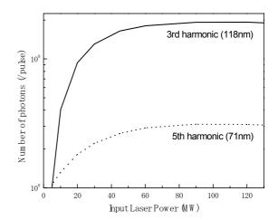
Figure 3: Calculation results of number of photons on the third and fifth harmonics as a function of the input laser power with the electron average current 1 mA.
