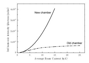
Figure 5: Expected number of photons for the new and old vacuum-chamber system as a function of the average beam current in one bunch ring operation.
