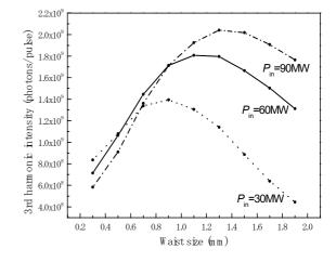
Figure 2: Dependence of the third harmonic intensity on the radius of the optical beam waist at the input laser power  $P_{\rm in}$ =30, 60 and 90 MW with the electron average current 1 mA.
