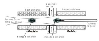
Figure 1: Schematic view of the setup for Coherent Harmonic Generation (CHG).
