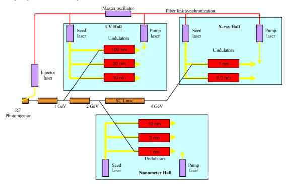
Figure 1: Layout of the MIT x-ray laser facility.
