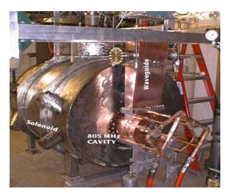
Figure 2: Solenoid and 805 MHz RF cavity
