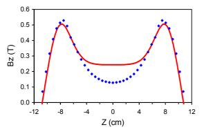
Fig. 2. Axial magnetic field profiles for the "volume" (solid) and minimum-*B* (dotted) configurations.
