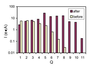
Fig. 5. Comparison of charge-state distributions for Ar ion beams extracted from the conventional minimum-B configuration before and after improvements made to the source.
