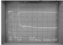
Figure 10 Output current  $i_0$  (4A/div), and output voltage  $v_0$ (100V/div) for  $i_0$  near zero for rated value of  $i_0$
