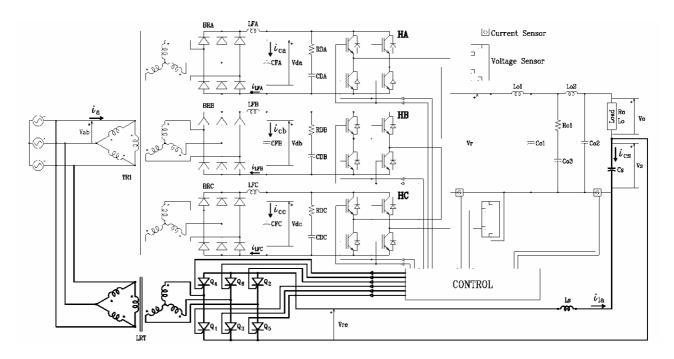
Figure 1 Basic 1,400A, ±900V Converter System with Energy Storage Capacitor CS and Six Pulse SCR Rectifier
