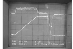
Figure 7 Output voltage  $v_o$  (100V/div) and output current  $i_o$  (400A/div)
