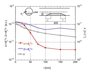
Figure 5: Intensity of axial magnetic field at downstream and upstream side,  $D-\langle B_z^2 \rangle$  and  $U-\langle B_z^2 \rangle$ , and the loss factor, k, as a function of the ramp length, l [mm], of a trapezoidal HOM source as sketched in the figure.
