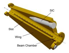
Figure 1: Structure of winged HOM damper.
