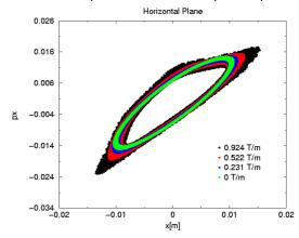
Figure 2: Horizontal phase space ellipses at one location of the ring after tracking for 62530 turns with different sextupole strengths. The nominal sextupole strength of 0.522 T/m is represented by the red ellipse
