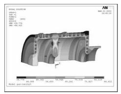
Figure 4: Temperature distribution in <sup>1</sup>/<sub>4</sub> of the guncavity when operating at an input power of 100 kW.
