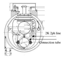
Fig. 5: Cross section of the TESLA cryo-module. The 2-phase-LHe line and the connection to the LHe-bath cryostat will be modified for CW operation.
