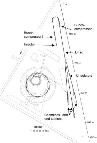
Fig. 1: Overview on the FEL adjacent to the present 3<sup>rd</sup> generation SR-source BESSY II operational since 1998.
