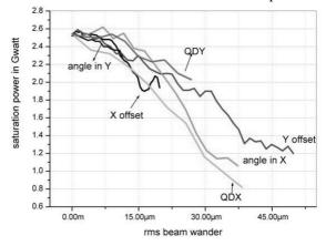
Figure 3: Influence of beam wander on saturation power caused by horizontal and vertical quadrupole misalignment (QDX, QDY), electron beam position offset (X offset, Y offset) and angle error (angle in X, angle in Y) at the undulator entrance. Calculations apply for the HE-FEL.
