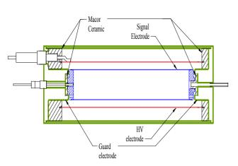
Figure 5. The new SNS ion chamber design.
