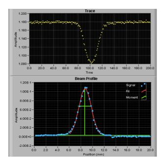
Figure 3. Horizontal beam profile in the SNS MEBT, measured January 2003. Top: an example of the electron collector signal. Bottom: the results of the measurement, with a Gaussian fit plotted out to  $2.5 \sigma$ .
