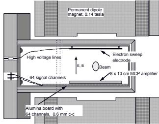
Figure 7. The original design of the SNS and RHIC IPM.
