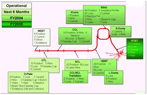
Fig. 1. Layout of the diagnostics in the SNS facility, color-coded to indicate the staged installation dates. \*Work supported by the Office of Science of the US Department of Energy.
