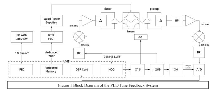
information is used to adjust the kicker power, compensating for variations in the beam transfer function portion of the loop gain. Overall system control is accomplished via a LabVIEW user interface.
