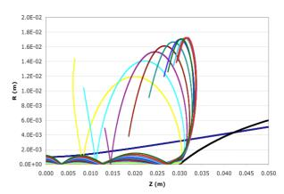
Figure 3: Surface which "bounces" ions out of beam
