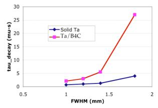
Figure 4: Decay time for composite vs. solid Ta.
