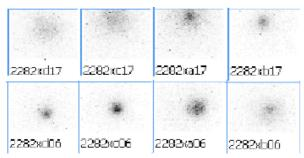
Figure 1: Time evolution of ETA-II X-ray spot with ions, for large (top row) and small (bottom) initial beam sizes.
