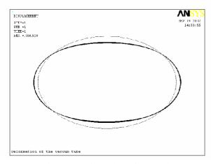
Figure 2. Deformation of Beam Pipe
