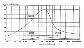
Fig. 2: Influence of dissolved oxygen on copper release rate. [20]
