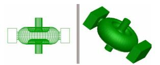
Figure 4: 1.5 GHz RF deflector model
