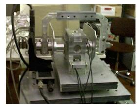
Figure 2: BPM calibration bench
