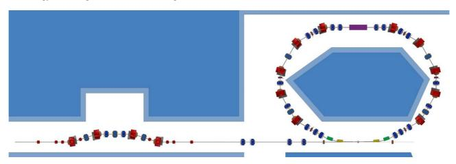
Figure 1: Layout of the Delay Loop and Transfer Line magnetic elements.
