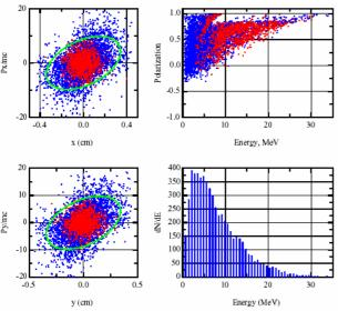
Fig. 2. (Blue) initial distribution of positron generated by 10.7 MeV  $\gamma$ -flux, (red) positron accepted at 1.9 GeV, (green) area of 0.03  $\pi$  m rad.
