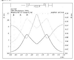
Figure 2: Lattice Functions in One Arc Cell
