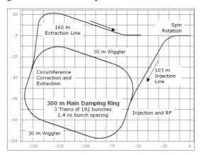
Figure 1: Overall Layout of the Electron MDR
