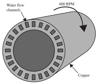
Figure 3: Schematic cross-section of beam dump cylinder design.
