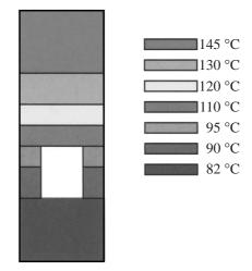
Figure 4: Calculated temperature profile in a dump cross section (20 °C water).
