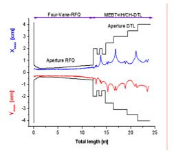
Fig. 4: 100 % transverse beam envelopes along the whole linac (RFQ+MEBT+H-DTL) in the nominal case.
