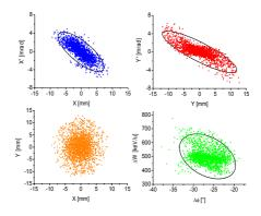
Fig. 7: Output distribution of the linac at 40.1 MeV with combined errors of the MEBT and H-DTL, 2000 macro particles used.
