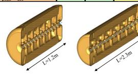
Fig.3: 3D view of the first and last 175 MHz sc CH-cavities (tank 1 and 4) calculated with MicroWave Studio®.
