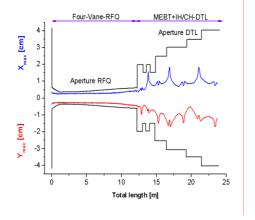
Fig. 6: 100 % transverse beam envelopes along the linac with combined errors for the MEBT and H-DTL.
