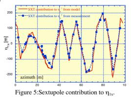
Collider operation has shown that the reduction of  $\eta_{1x}$  is beneficial for dynamical aperture and beam-beam behaviour, since the best luminosity results have been obtained after cancelling, almost completely  $\eta_{1x}$  in the KLOE IR (IP at 25.72 m), see Fig. 6.
