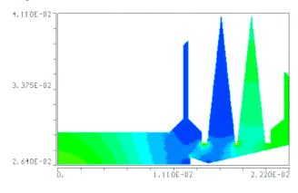
Figure 5: Dipole 5.46 GHz. Magnetic energy density.
