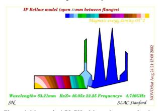
Figure 4: Monopole 4.75 GHz. Magnetic energy density.
