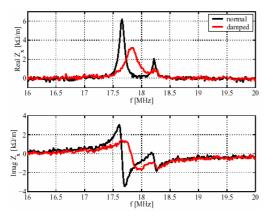
Fig. 3. Transverse impedance of the RF cavity
