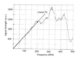
Fig. 2 -  $B_{\theta}$  measured inside wire mesh at r = 4.625".
