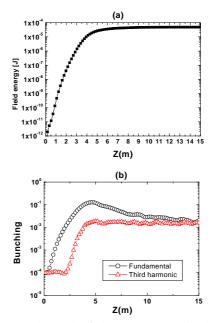
Figure 5: (a) shows the field energy at the fundamental. (b) shows the bunching fraction for the fundamental and third harmonic.
