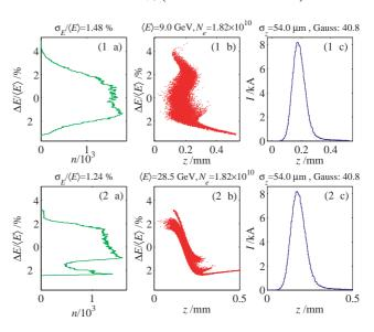
Figure 2: Beam at chicane exit (top) and end of linac (bottom), showing longitudinal phase space (1-b & 2-b), energy (1-a & 2-a), and temporal (1-c & 2-c) distributions (gaussian-fit in red:  $\sigma_z \approx 40~\mu \text{m}$  rms).
