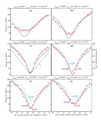
Figure 3: Wake-loss scans (the vertical scale has an arbitrary offset) with varying  $V_{RTL}$  from 40 to 45 MV, (a) to (f), respectively. The 42-MV case (c) also plots the simulated rms bunch length: scale at far right.
