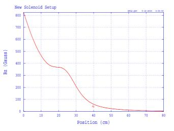
Figure 2: Bz from new solenoid setup
