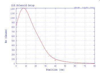
Figure 1: Bz from old solenoid setup
