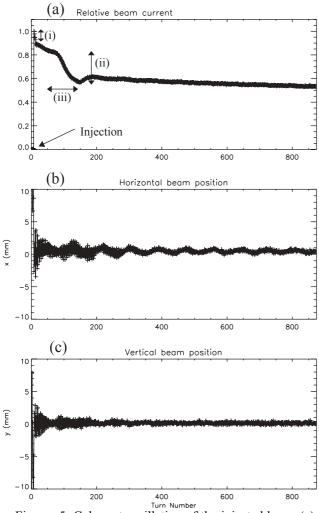
Figures 5: Coherent oscillation of the injected beam:(a) shows the turn-by-turn relative beam current, (b) the horizontal beam position and (c) the vertical one. The horizontal axis indicates the turn number from the injection.
