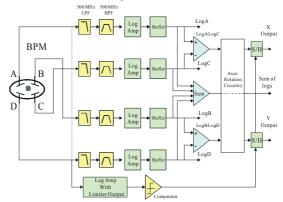
Fig. 1: The block diagram of the turn-by-turn beam position measurement system.
