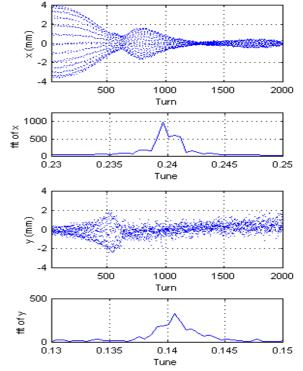
Fig. 2: The measured horizontal and vertical turn-by-turn beam positions at resonance of  $3v_x + 2v_y = 30$ . The corresponding tune spectrum is shown under its beam position spectrum.
