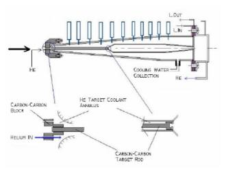
Figure 1: Sketch of First Horn with target inserted.
