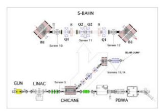
Figure 2. UCLA Neptune beamline with S-Bahn.
