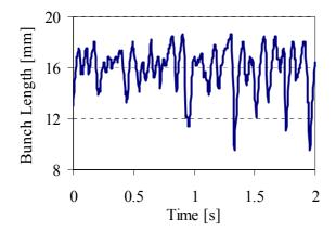
Figure 6: Bunch length vs. time of a 15 mA beam excited by a longitudinal mode at 500 MeV.
