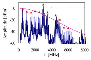
Figure 2: Beam spectrum. Markers point out the harmonics of the RF frequency.
