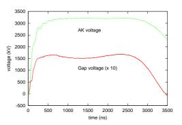
Figure 2: Voltage pulse applied to AK gap (green) and to accelelerating gaps (red). The latter has been multiplied by 10 for scaling purposes.
