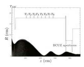
Figure 1: Geometry of desorption calculation, showing injector, 8 accelerating gaps, and BCUZ. The beam is shown at the flat-top energy and current.
