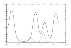
Figure 5: Ratio of ion  $(H_2O^+)$  charge to beam charge vs. z at t=1000 ns, within a radius of 1.5 cm (red line). The axial solenoidal magnetic field in kilogauss is overplotted (black). Horizontal scale is in cm.
