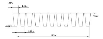
Figure 7: Tune modulation of particles in the center of a bunch due to moving collsion points, for  $\Delta f_{rf}=5$  Hz, no crossing angle, 60 bunches and a total beam-beam tune shift of  $\Delta Q_{tot}=-0.005$ .
