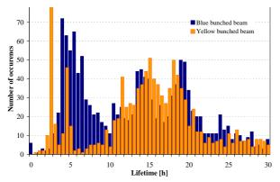
Figure 3: Blue and Yellow bunched beam lifetimes with proton-proton collision during one month of operation.
