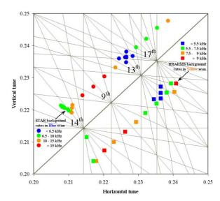
Figure 4: Experimental background rates as a function of fractional tunes. For these measurements deuterons in the Blue ring collide with gold ions in the Yellow ring. The total beam-beam tune spread due to the beam-beam interaction is about  $\Delta Q_{tot}=0.005$  in both measurements.
