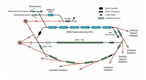
Figure 1: Schematic Layout of 4GLS Light Source Concept
