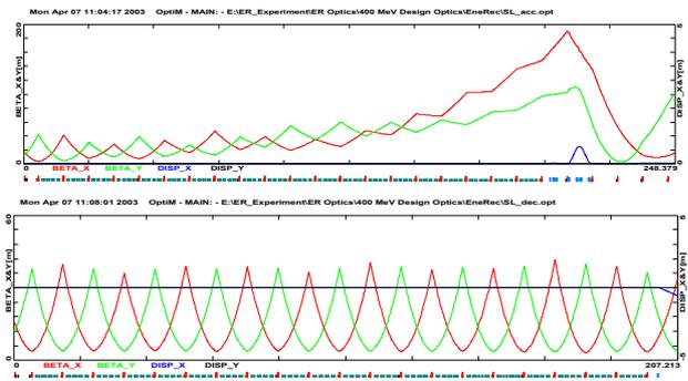
Figure 3: South Linac – top: mismatched optics for the accelerating beam (556–1056MeV) and bottom: 120° per cell lattice for the decelerating beam (556–56MeV)
