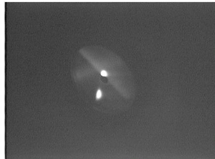
Figure 5: Two beams (~ 1 GeV and ~ 100 MeV) at the end of South Linac - SL16 beam viewer ( $E_{inj} = 20$  MeV)
