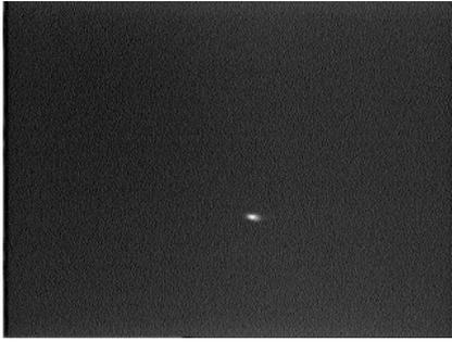
Figure 6: Energy recovered beam (56 MeV) at the dump (optical transition radiation monitor view)
