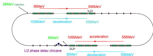
Figure 1: CEBAF Energy Recovery Experiment - layout
