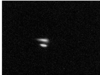
Figure 4: Arc1 synchrotron light monitor – two ‘spots’: accelerated/decelerated beams at 556 Me
