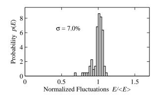
FIG. 3: Histogram of HGHG output pulse energy with 30MW seed power
