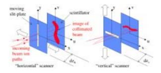
Figure 6: Schematics of "optical slit" scanners.
