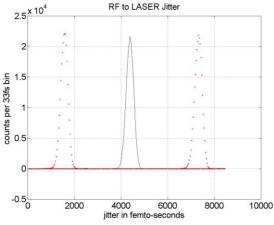
Figure 5. Laser to RF jitter in an 8 second histogram length with +/- 3-degree calibration traces.
