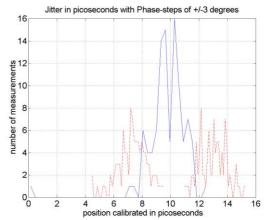
Figure 3. Beam jitter as measured by position on YAG screen after spectrometer magnet.
