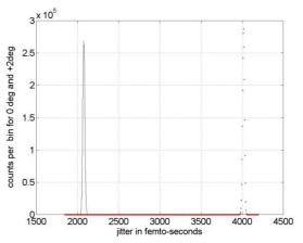
Figure 6. Laser to RF jitter in 8-second histogram length when RF is driven by laser output. A +2-degree calibration trace is on the right, second calibration trace omitted to improve scale for clarity.
