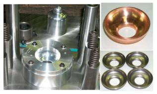
Fig.3. Tooling. Copper and niobium half-cells.
