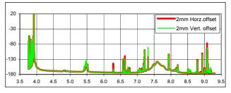
Fig.9. Field amplitude in cavity (dB) vs. frequency (GHz).
