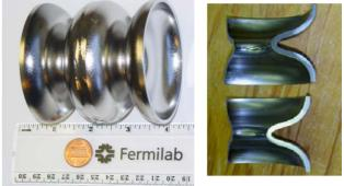
Fig.5. Welded dumbbells
