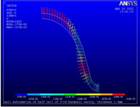
Fig.2. Distribution of surface displacement.
