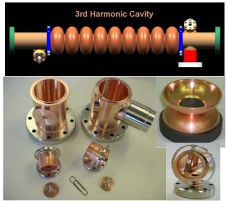
Fig.7. Cavity, end-tubes, dumbbells and HOM couplers.
