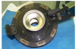
Fig.6. Frequency tuning device.
