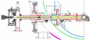
Fig. 8. Coaxial input coupler.
