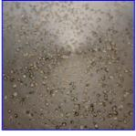
Figure 2: Cu window after RF conditioning with the external 2.5 T magnetic field in solenoidal mode. Surface damage (pitting) can be seen clearly on the photo (right), which is a close-up view of the center region of the same window.
