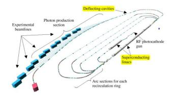
Figure 1: The layout of the proposed LUX machine
