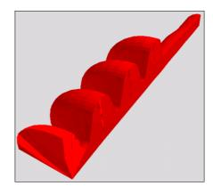
Figure 4: 3-D MAFIA model for the 7-cell deflecting cavity (1/4 of the structure shown here)
