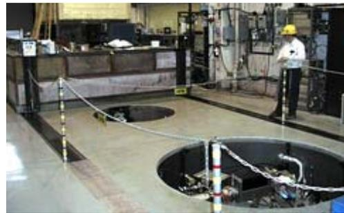
Figure 1: Test pits for various size cavities. Shown is the small and the large pit. Not shown is the medium size pit.
