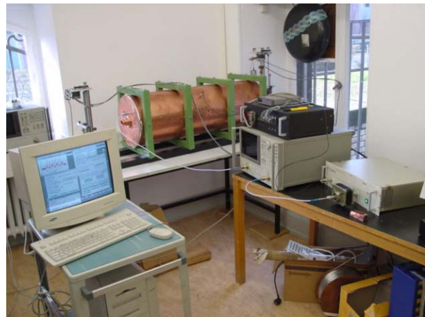
Figure 3: Photograph of the experimental setup. In the center the CH r.t. model is visible.
