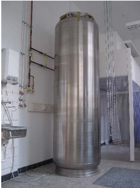
Figure 6: The 3 m long vertical cryostat (center) and the class 100 laminar flow box (right) in the new cryogenic laboratory in Frankfurt.
