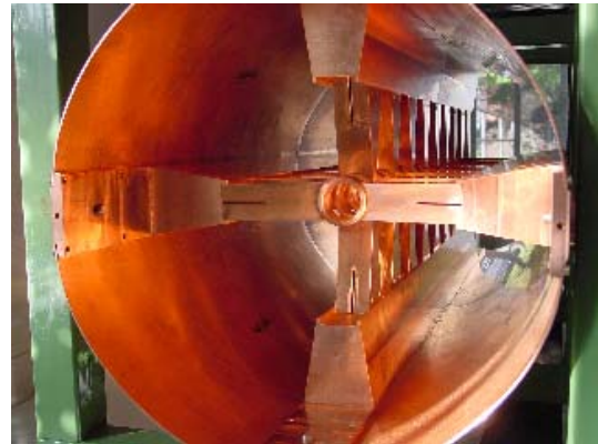
Figure 2: View into the CH copper model. The characteristic crossed stem construction of the CH cavity is clearly visible.
