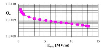
Figure 4:  $Q_0$ - $E_{acc}$  curve at 2 K of the Q-degraded cavity EZ02. This cavity was held at 100 K for a total 180 hours. The  $Q_0$  at the lowest measured  $E_{acc}$ =0.37 MV/m was 4.54E9, which was still lower than the initial value of ~6E9 of the non-degraded cavity.
